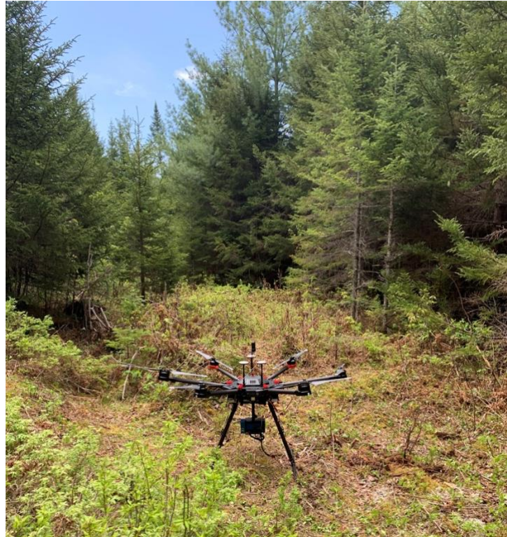
Drone, equipped with LiDAR sensor, ready for takeoff at one of our low elevation sites in the White Mountain National Forest.
